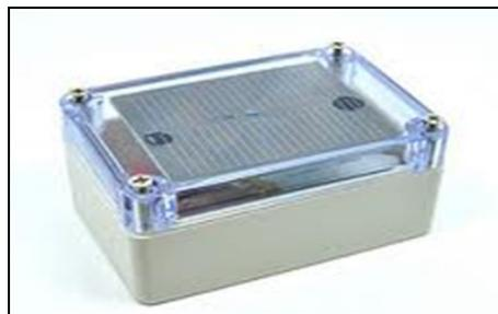
**Deliverable:** Solar Reporter – a remote terminal data logger unit that can measure, and data-log the temperature, humidity and generated current at the solar PV farm.
