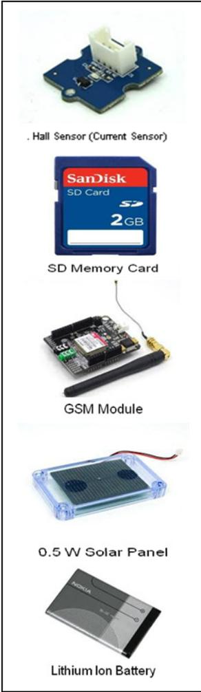
iii. **Hall current sensor** – This is a non-contacting current sensor that can measure the current generated by a solar PV panel. The data is then sent to the micro-controller.
